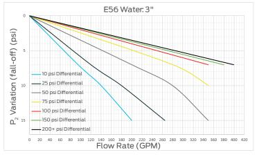
$\textbf{Pressure Differential:} \ \textbf{Difference between the inlet pressure and the PRV set pressure.}$
